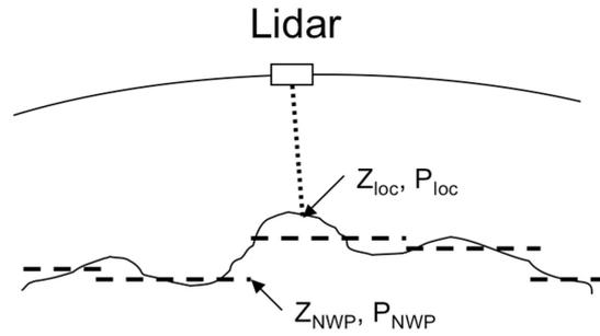
Figure 1.- Link between grid box elevations provided by NWP models, range and target altitude
